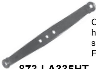
Category 1- Right or Left Lift Arm - Made of 1/2" x 2-1/2" alloy steel has 7/8" pin holes on both ends, 31-3/4" ball centers, and overall length is 34-1/4". Center section is heat-treated. Fits Ferguson, all models; Ford 2N, 9N, 8N, NAA; Massey Ferguson 35, 50; Oliver 550 and Oliver 3-point conversion; John Deere 1010.
